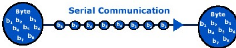
Fig3: Serial transmission used for long distance communication.
